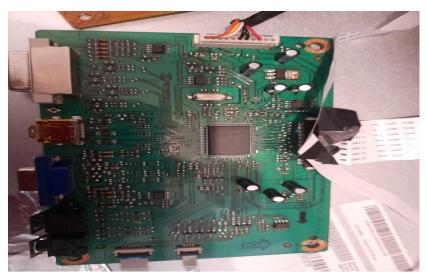
This is the monitor controller, this is the heart of the monitor, it takes the signal from the HDMI or VGA cable and translates it to a signal that the monitor can read. It controls the brightness, colour and contrast of the screen. The controller also has an output and input for audio because HDMI also sends audio through the cable.
