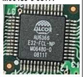
USB2.0 Single LUN Multiple Flash Card Reader Controller The AU6366 reads and processes the data inputted from the CF Card Slot (which is connected to the daughterboard).
