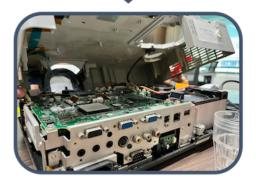
Lifting the cover off and removing the wires connected to the case to reveal the inner workings of the projector
