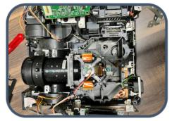
The deconstructed projector's optical engine
