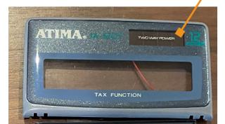
contains a solar panel that extends the calculator's life by recharging the main battery. Solar cells (photovoltaic cells) take the sun's energy to emit electrons through a process called the photoelectric effect. When sunlight shines on the solar panel, photons hit the silicon atoms and transfer energy to the electrons. Two silicon elements, the n-type (positively charged) and p-type (negatively charged), are created, forming an electric field for the calculator to power.
