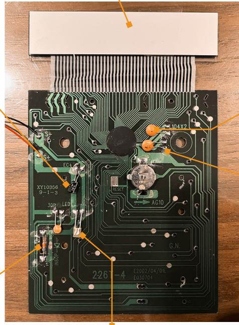
The ceramic layers within the two ceramic disk capacitors are dielectric. Their efficiencies are at 100,000 pF and 30pF.
