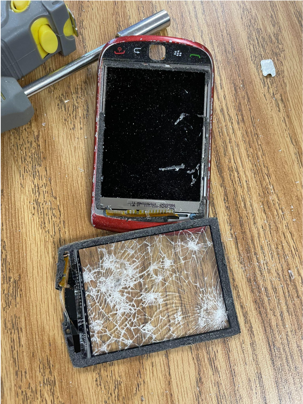
The touch screen, and the glass cover.
