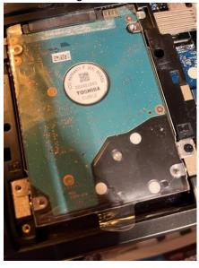
After removing the three screws holding it down, I had to slide it out of place.
