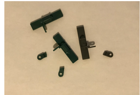
Figure 1. Broken conveyor-belt base links and tank treads.
