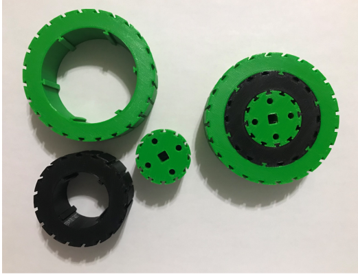
Figure 11. Two 3D printed finalized Onion Rollers, which includes a separated Onion Roller (left) and a maximum sized Onion Roller (right).
