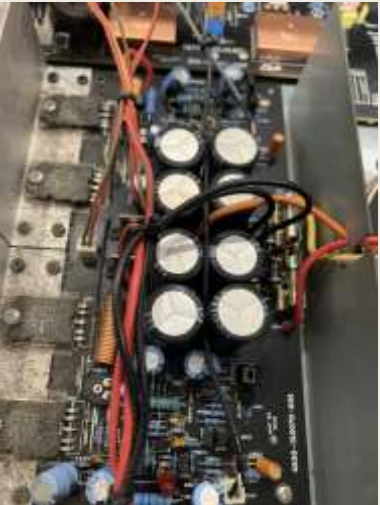
Capacitors - stores small amount of charge quickly
