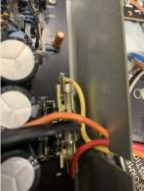
Diode - Ensures electricity only flows in one direction
