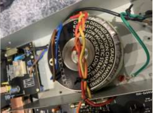
Transformer - transforms the 220-240v to its necessary voltage
