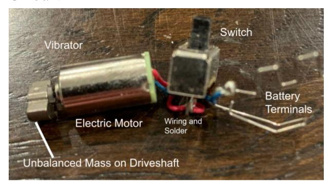
This circuit is the base of the entire HEX bug. When the switch is flipped it connects the battery terminals to the vibrator. The electrical motor then spins its driveshaft. Attached to the driveshaft is an unbalanced mass which when spun very fast causes the motor to shake or vibrate, and since the motor is very tightly secured inside the body of the bug the entire bug vibrates along with it.
