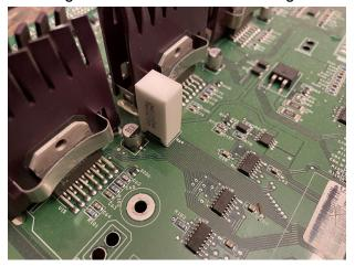
The test points are directly above the motor drivers. The printer has a 3x16 character LCD, but it is very limited for all the systems to monitor on this printer, so the makers of the printer had a solution: measure voltage at these terminals manually.
