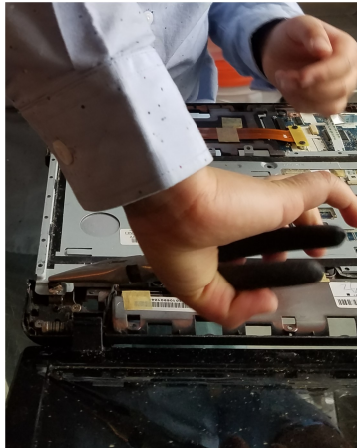
Figure 4: Using pliers to remove the DVD drive
