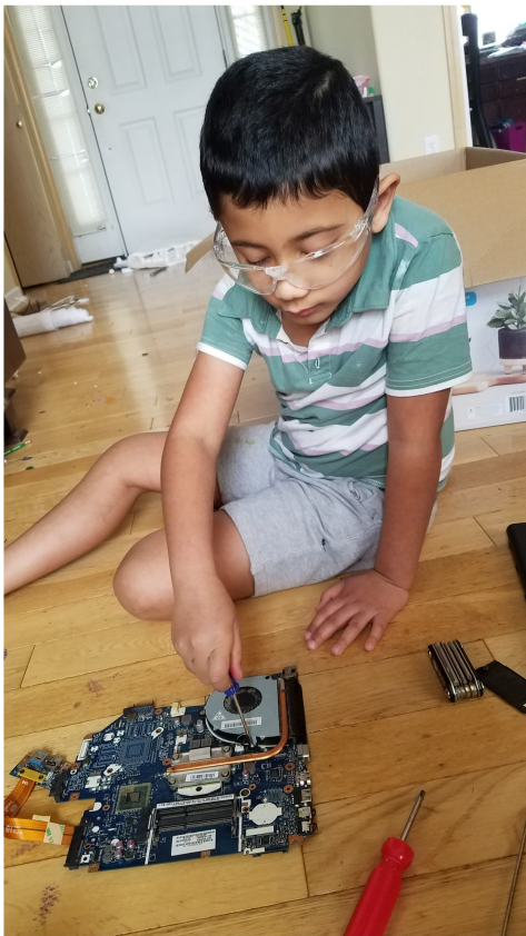
Figure 1: Unscrewing the heat sink (top) and fan (bottom)
