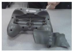
Then we used a screwdriver to remove the handle/side, where we found the inside.
