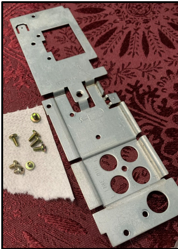
Figure 9: The outside wall on the opposite side of the radio panel, with eight screws.
