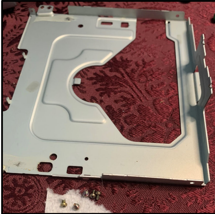
Figure 11: Exterior of the CD assembly where figure 7 rests, with five connecting screws
