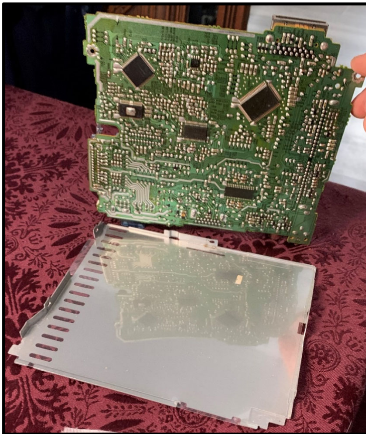
Figure 6: The plastic sheet is down on the metal. The green is the bottom of the motherboard. The metal is part of the metal frame walls
