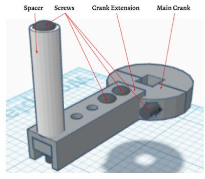
by shrinking a cylinder and adding a square hole in the middle. I then made a rectangular prism for the extension by adjusting a cube. Next, I made the extension by making a slightly larger rectangular prism. I copied and pasted the main crank's rectangular prism, and made the copy a "hole" piece and cut out a section for the crank extension.
