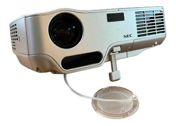
The NEC NP60 Projector is 2.90" x 9.70" x 7.10", and is 3.5 lbs with a resolution of IO24x768. It has an audible noise of 40 dB and is 285 Watts IOOV - 240V. It uses Digital Light Processing (DLP) technology and is an 8-bit color processing projector.
