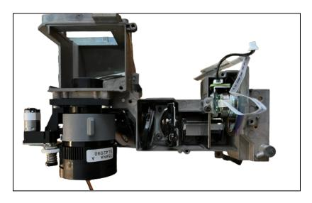
The color wheel (right side of image) is a constantly spinning glass disk with different colored sections. The DLP chip coordinates the DMD mirror direction with what colors are being directed towards the DMD. As the different colors are reflected on to a screen, our brain merges these quickly changing colors to be one color.
