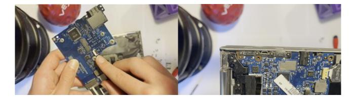
[6:15] Screwed onto the motherboard was a <u>Local Area Network chip</u>, which allows a device to connect to other devices locally. Underneath was the date the circuit board was made 11<sup>th</sup> December 2017.
