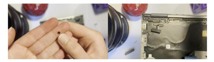
[11:18] The keyboard remained, which took a while to remove due to many screws. Once off, I could see how the keys worked and removed all keys.
