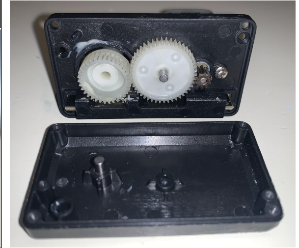
The previously mentioned gear train, connecting the internal motor's output (metal gear) to the plastic output gear that interfaces with the cartridges.
