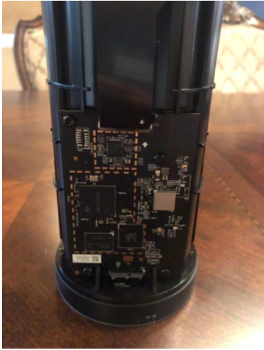
Figure 1.9: Amazon Echo with system board.
