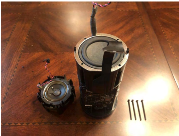
Figure 1.7: Amazon Echo with woofer removed.
