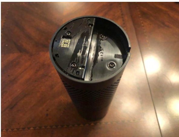
Figure 1.3: Upside down Amazon Echo with rubber base removed.
