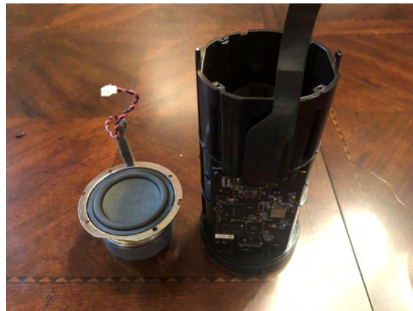
Figure 1.8: Amazon Echo with tweeter removed.
