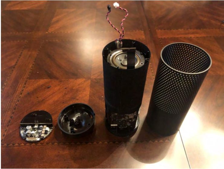
Figure 1.5: Amazon Echo with power board and outer casing removed.
