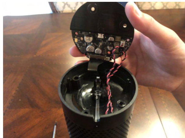
Figure 1.4: Amazon Echo with 4 long screws removed, and power board being removed.
