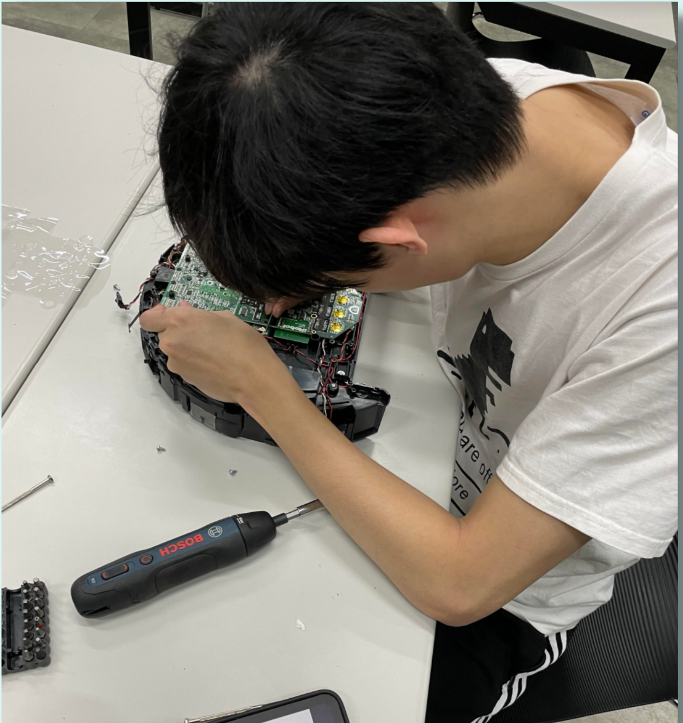
Our builder dissects an iRobot Roomba 880 to learn more about its circuit boards and chips.
