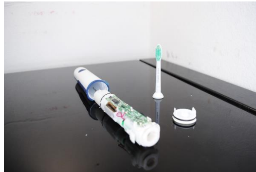
A) Separation of the two main components: head brush and brushing mechanism.
