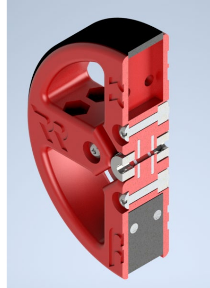
Renders of the Custom Traction wheel showing the integrated bar locks and tread attachment mechanism.
