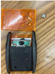
Figure 3: The back of the calculator has been removed. The battery has been removed and we can see two red wires connected to the circuit board.
