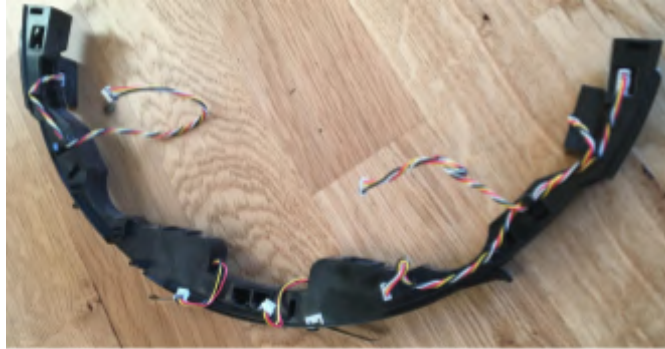
Fig 5.2 The front sensor board assembly
