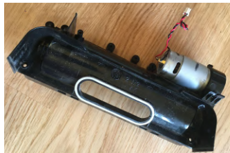
Figure 3.10 The disassembled brush motor and vacuum chamber entrance
