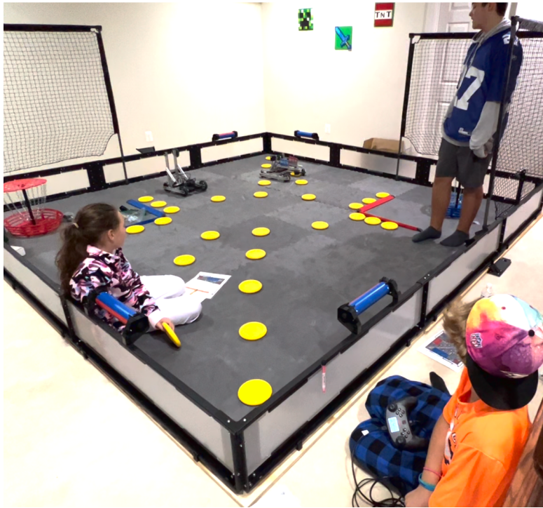
Figure 10 Failing a test because discs are pushing our robot off course and over the autonomous line
