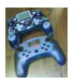
I began by taking off the 8 screws that connect the top and bottom of the controller.
