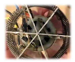
a. Mica paper contains the heat from the coils to keep the outside plastic from melting from the coils.
