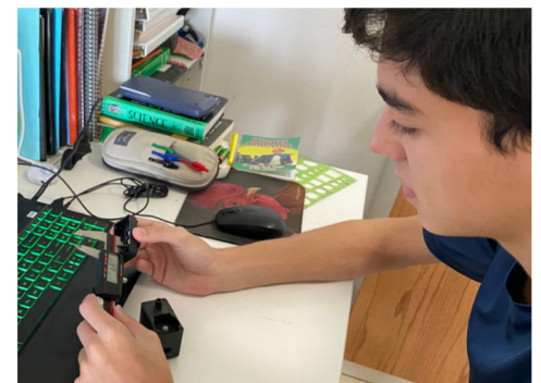
Figure 10: Measuring motor cap with a caliper
