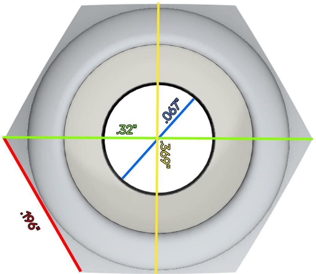
Fig. 3: A Diagram of the Pneumatic Locknut
