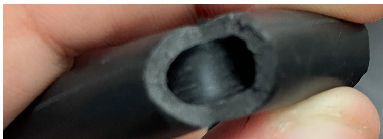
Pictured above is a section of the air tubing with no problems
