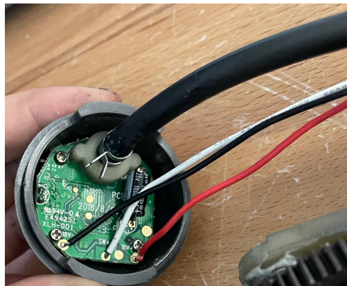
Pictured above is the connection point between the air tubing, the pressure sensor, and the LCD
