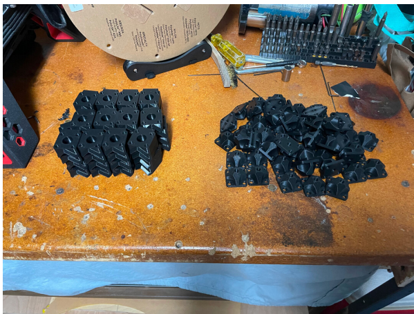
(a) Printing the roller molds
