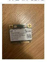
The WLAN (Wireless Network Interface Controller) card is a network interface controller card which connects to a wireless network, such as Wi-Fi or Bluetooth, rather than a wired network, such as a Token Ring or Ethernet. It makes the laptop portable and able to be taken to many places, without needed to be physically connected to the internet.
