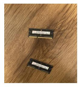
The RAM consists of 2 2GB sticks. The RAM allows for more tasks to be run simultaneously on the computer. It can be accessed by screwing off a panel on the bottom of the device, which makes it easy to replace.
