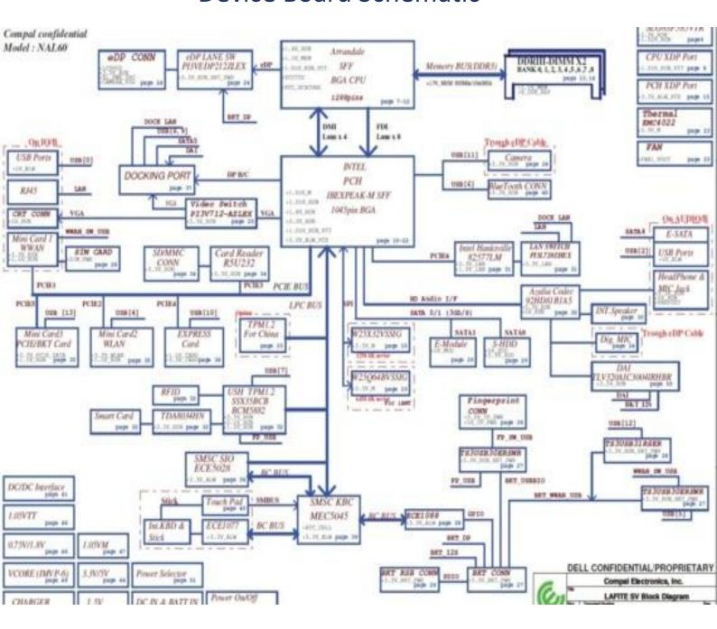
This is the schematic that we used to identify all the components and the motherboard. It shows how different parts interact with each other to create a successful system.
