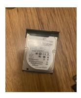
The storage drive which this computer utilises is a 256 GB 7200 rpm (how many times it spins a minute) HDD (Hard Disk Drive). This is used to store media
