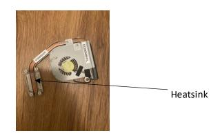
The fan lies on the edge of the motherboard and the heatsink leading to it screws directly above the processor, so that it can take heat away from it to keep it cool for better overall performance.
