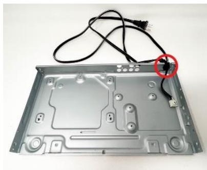
Figure I 8. Snap off power cord from the bottom chassis
