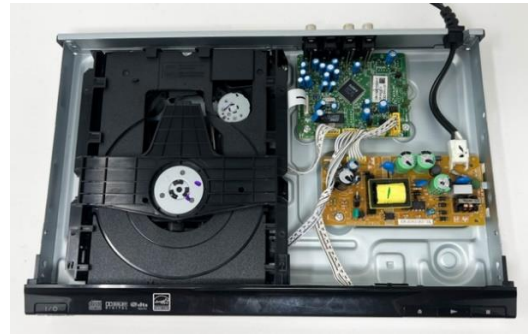
Figure 5. Remove top panel, exposing subcomponents
