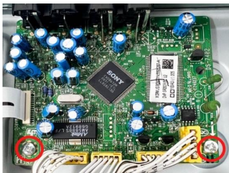
Figure 8. Take out 2 screws from Board 2
