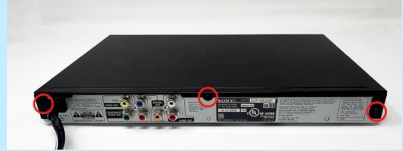
Figure 3. Take out three screws from back panel
