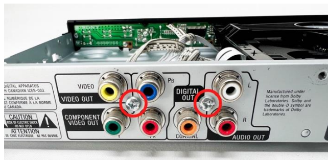
Figure 9. Take out two back panel screws from the rear panel
