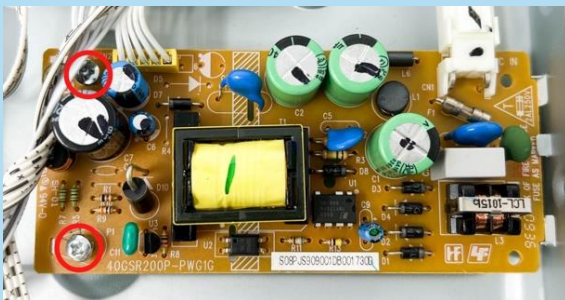
Figure 6. Take out 2 screws from Board I
