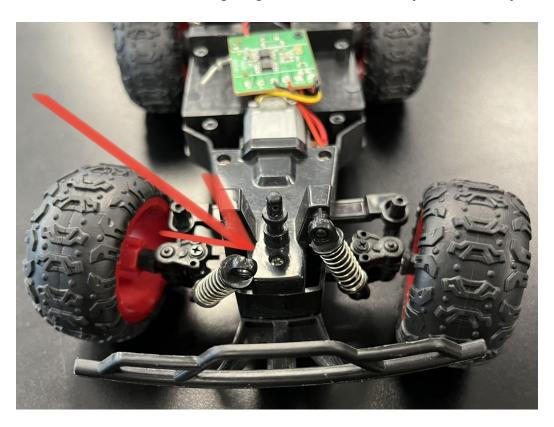
Step 5: We took out all the screws holding the wheels on. Then we removed the wheels. Doing this task will make it easier for us to access the rest of the car.
