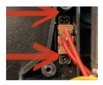
Step 10: This is when we will disconnect the rear motor module. Two screws held a bracket holding the rear motor module, and then we lifted the module.
