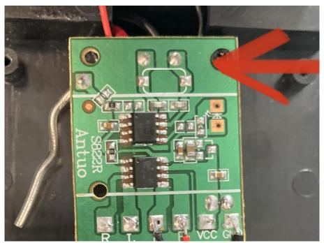
Step 9: This is where we took out the On/Off switch and two screws held onto it. After this, we could fully take out the circuit board, servo, and switch.
