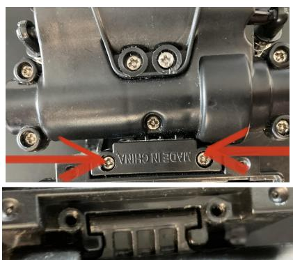
Step 11: Once you pulled out the motor module, we needed to unscrew all nine screws holding the rear motor module together.
