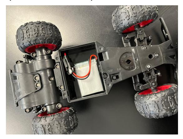
Step 2: Next, we flipped the car and took out the top three pins holding onto the car's shell.
