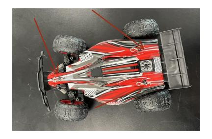
Step 3: We took out the four screws covering the circuit board.
