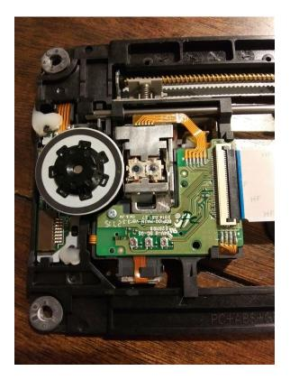
Assembly Deck: The Assembly Deck contains the main components of the DVD player. Some of these parts include the tray, disc drive motor and gears. The tray is a thin plastic disc holder that allows a CD, DVD, or Blu-ray disc to be inserted into the computer. The disc drive motor makes the gears spin, rotating the disc in the tray.
