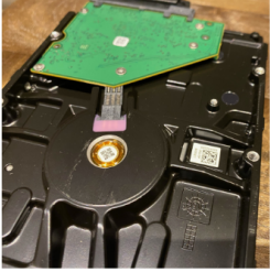
Back of HDD, circle is the middle of the platter
