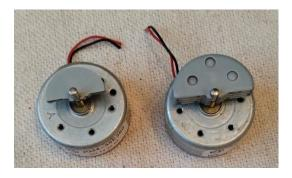
6. Lastly, we took out the vibration motors from the internal bracket grooves by pushing them out of the grooves with our thumb.
