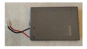
2. We unplugged the battery's connection from the motherboard and removed the battery to ensure that there is no electricity in the components for safety purposes.
