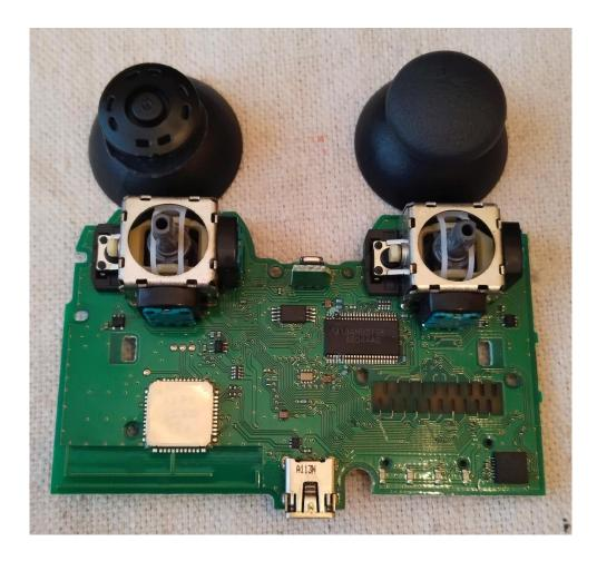
The Analog Joystick, sometimes called a control stick or thumb stick, is an input device for a controller that is used for twodimensional input. One of the sticks is used for the vertical movement (Y-axis) and other for the horizontal movement (X-axis).
