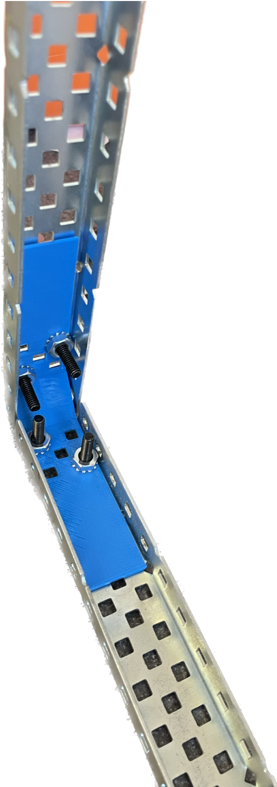
This is the L bracket inside of the c channel
