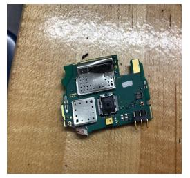
(A piece of the motherboard broke off) The motherboard is the central circuit that connects all of the components and allows them to communicate with each other. Wires are soldered onto the motherboard so that all the individual components are connected to each other. With all of these different parts, the capability of the circuit board is expanded.
