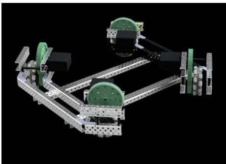
A rendering of our chosen solution, in this case the drive train, in Fusion 360.
