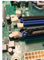
Figure 3.2.1.6 RAM Slot Clips
