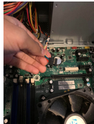
Figure 3.1.1 Detaching wires from power supply
