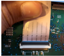
Figure 3.2.3.1 Disconnection of Optical Drive Wires
