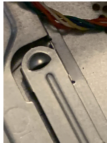
Figure 3.1.5 Lever Attaching Power Supply to Frame
