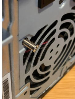
Figure 3.1.4 Detaching Screws Connecting Power Supply
