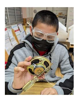
I discovered the speakers were magnetic when my screwdriver got stuck to one. Magnets make the speakers move which creates vibrations. The vibrations create the sounds we hear when we hear the music.
