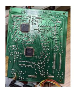
I saw a lot of silver spiky things on the circuit board. I found out that they were solder. My coach said you pronounce this like 'sodder'. This keeps the wires from the other side in place. Solder is an alloy that's melted to join metal objects.
