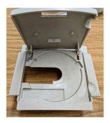
The lid lifts by a gear. The gear has an end, first with teeth than smooth. This keeps it from going too far back and breaking. On the other side of the lid is a spring. The spring holds the lid in place to keep it from falling back down.
