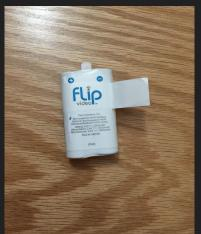
This is the batteries of the camera. It seems to be 2 rechargeable AA batteries conjoined together so they don't get lost and get charged together
