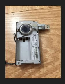
This is the 'case' of the camera that holds the screen, batteries, and the circuit board. It also has a USB stick attached to it so you can access the files in it.
