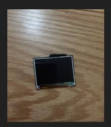
This is the screen of the camera. It is the output of camera as it shows what the camera is capturing. While assembling, it goes between the front cover and the 'case'.
