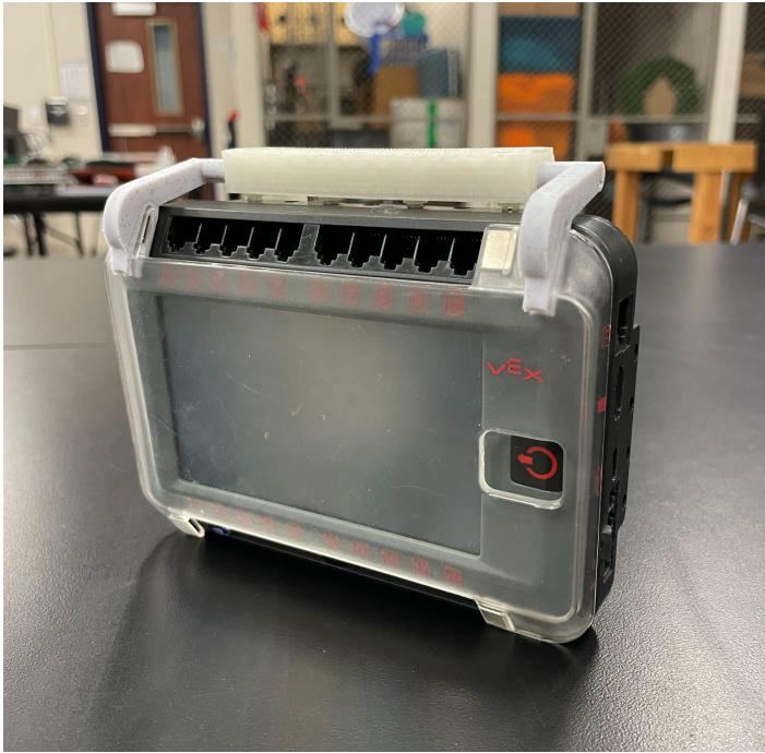
Images of 3D printed Cover Hinge on an actual brain and cover
