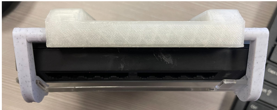
Images of 3D printed Cover Hinge on an actual brain and cover
