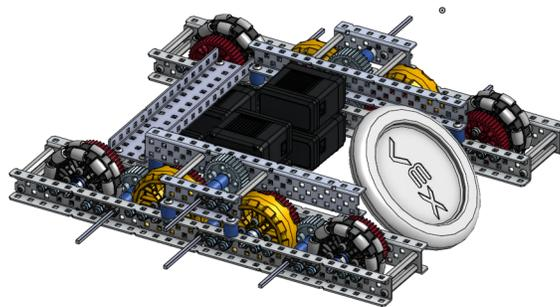
62880A V3 Drivetrain made using Onshape
