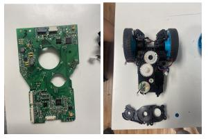
4. Separate wheels, motors and motor housings
