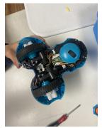
2. Unscrew more screws, take out the wires and then separate the motherboard from the shell along with wheels, wheel motors, and motor housings.
