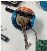
7. Split the dead shell into halves and take out head buttons and eye light board
