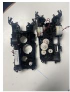
5. Separate speaker and infrared board from the bottom shell
