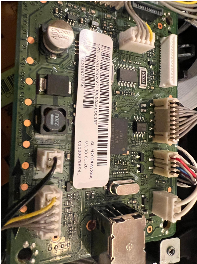
Supplementary board with data port connected on top of motherboard with flat wire connector
