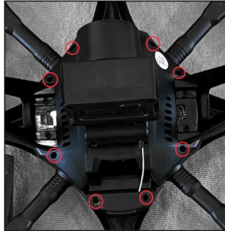
Figure 2.3 - the holes from which the screws were removed
