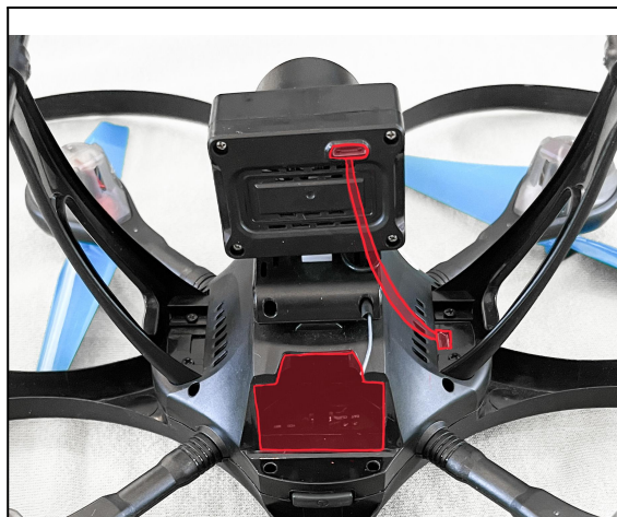
Figure 2.2 - the lower drone body, with now missing parts drawn in red
