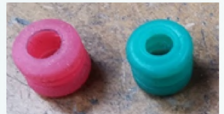
Shock absorbent spacers: Absorb vibrations of the movement of laser assembly
