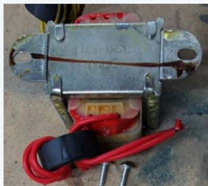
Transformer: Steps up voltage input to CD player
