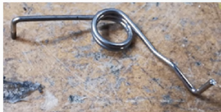
Opening spring: Uses its elastic potential to open CD cover when pressed
