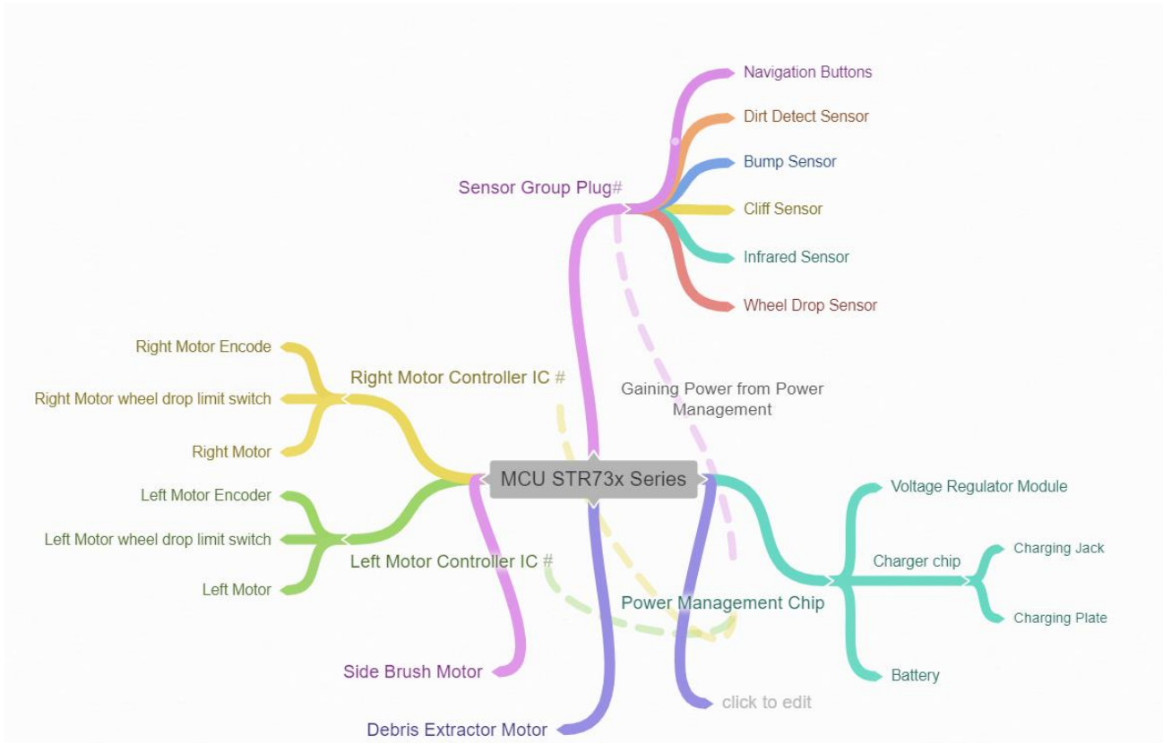
Figure 3.1: Architecture Diagram of iRobot Roomba 565
