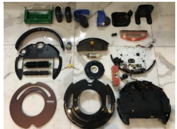
Figure 5.2 All components of Roomba
