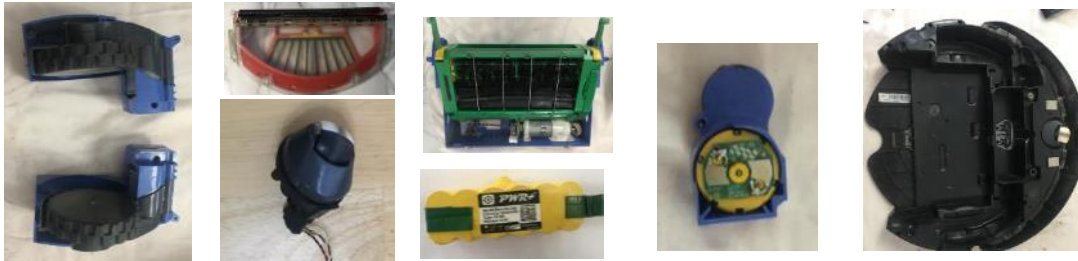
Figure 5.4: Parts located in the bottom side of the robot
