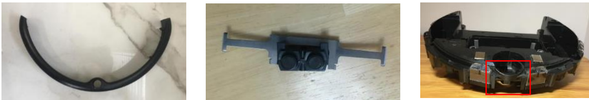
Figure 5.7: The robot’s collision detection
