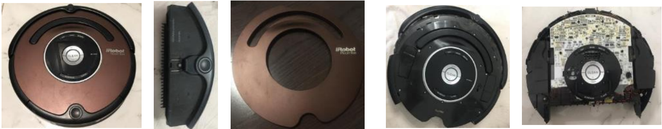
Figure 5.5: Taking off the robot’s top layer, revealing the motherboard
