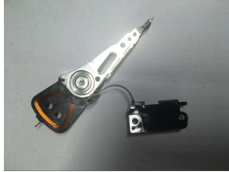
Fig 10 and 11 – The actual 6 drive heads and the control arm
