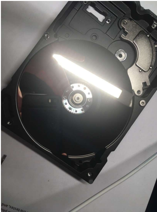
Fig 12 – Just the platters and motor in the drive housing
