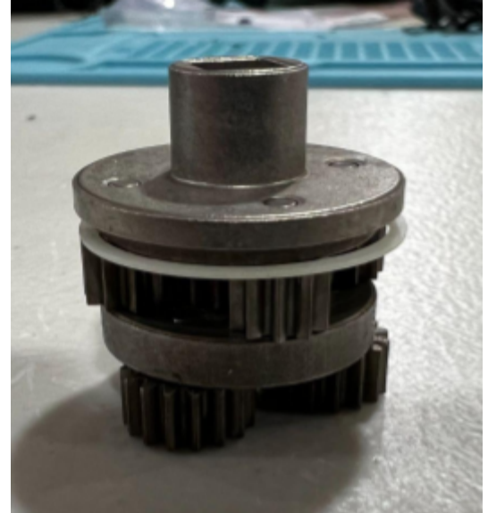
Fig 1: Gearbox of 18:1 Motor Cartridge
