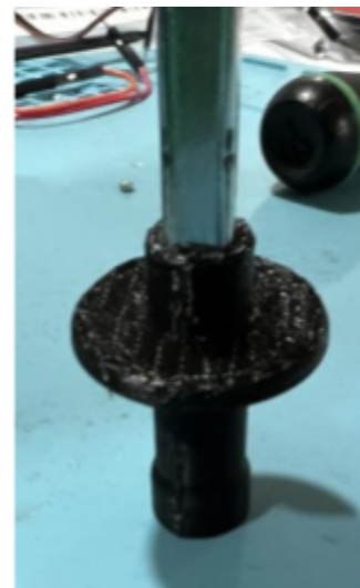
Figure 9: Stabilizer V1 with HS driveshaft
