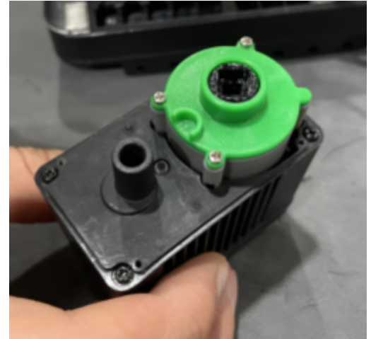
Figure 14: Assembled stabilizer in a motor
